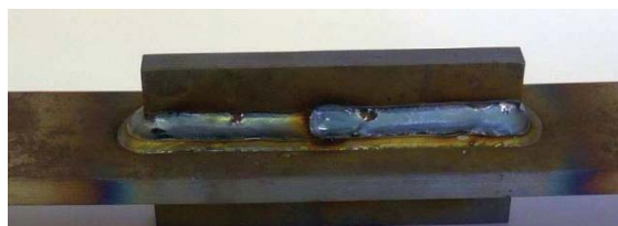
Figure 1 — Seam weld as 1-dimensional joint
