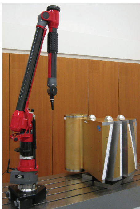
Figure 10 — Portable measuring arm with gear artefact
