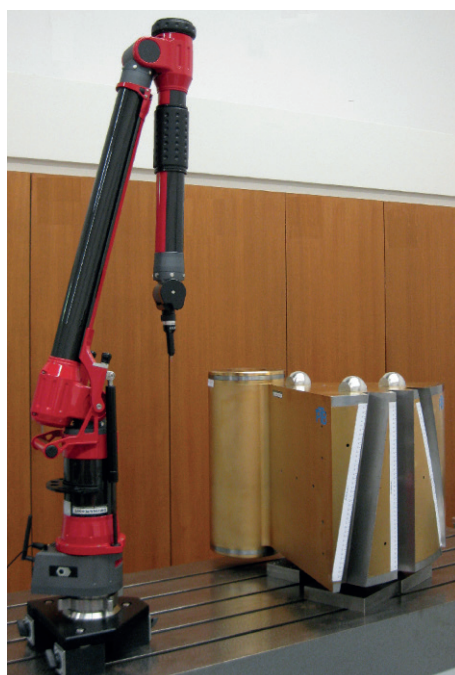
Figure 10 — Portable measuring arm with gear artefact
