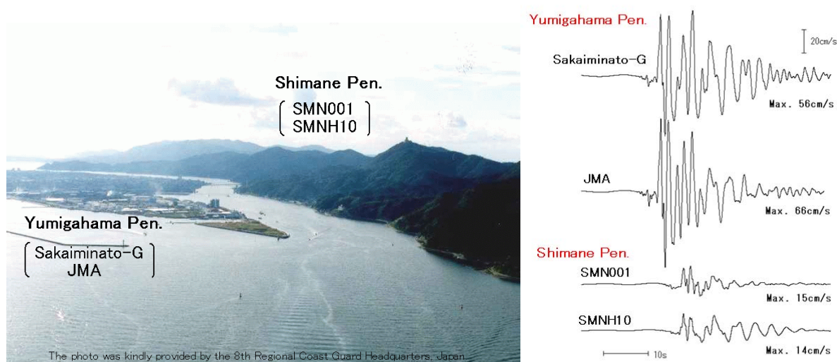
Figure 30 — The topography around the Port of Sakai, western Japan (left) and the velocity waveforms for the fault-normal component recorded around the port during the 2000 Tottori-ken Seibu earthquake (M J 7.3). The peak ground velocities observed in the plains of Yumigahama Peninsula were approximately four times larger than those observed in mountainous Shimane Peninsula (Nozu et al., 2008).
