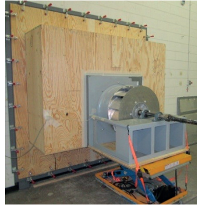
Figure 20 — Inlet cabinet with side wall spacings 1D right, 1D top and 1D left
