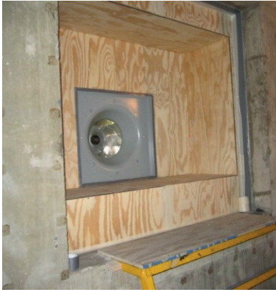
Figure 20 — Inlet cabinet with side wall spacings 1D right, 1D top and 1D left
