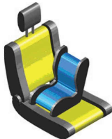
Figure 5 — Example of CRS wrongly positioned
