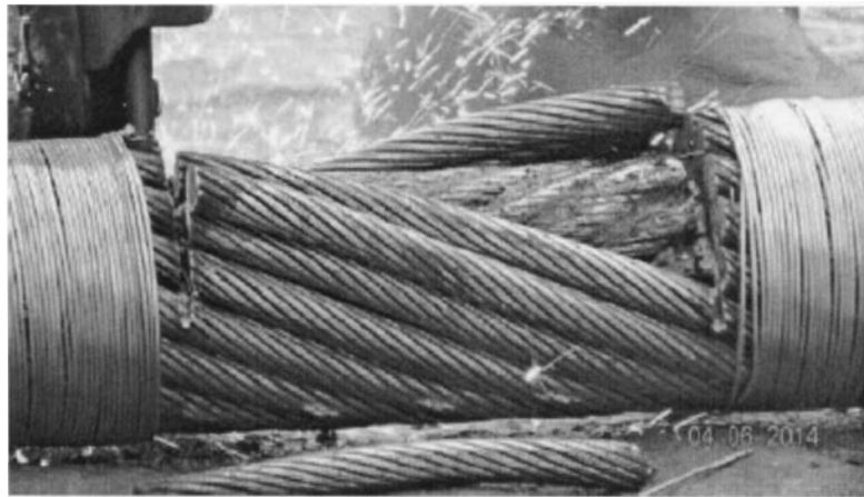
Figure 3 Alternative seizing and cutting method for large diameter rotation-resistant rope
