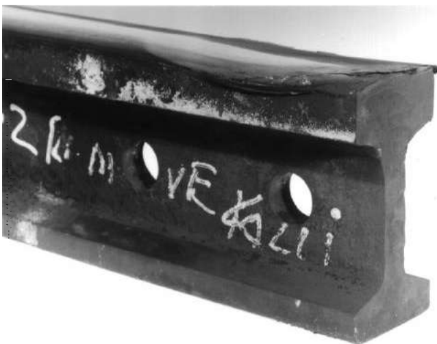
Plate 14 Rail end with severe crushing of the running surface
