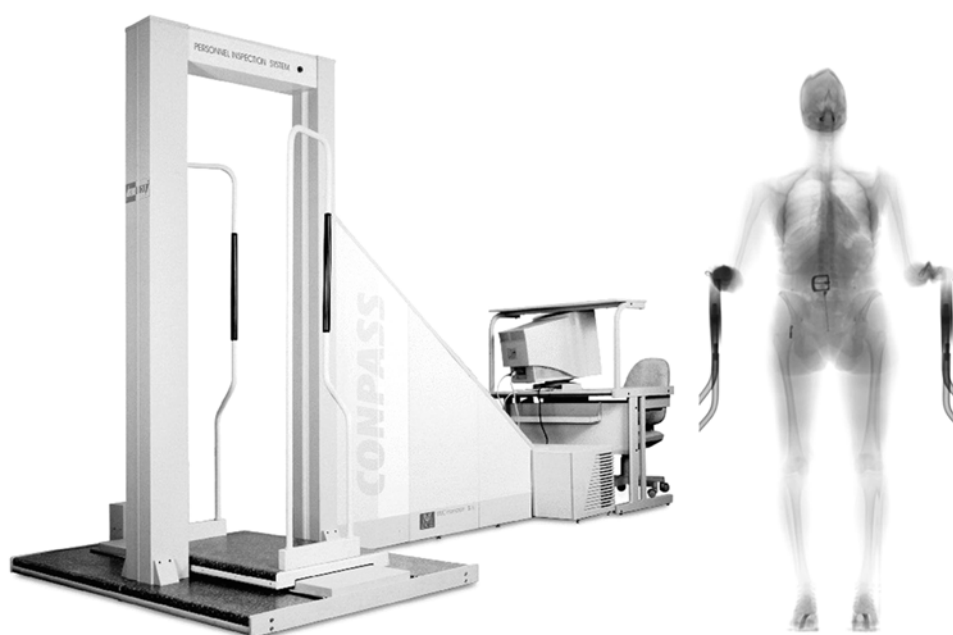
Fig. 1.4. The Compass® transmission system and sample image (photographs courtesy of X-Ray Equipment Company, Miami, Florida).
