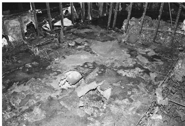
FIGURE 6.17.8.2.5(a) Fire Patterns on Floor Resulting from Fully Developed (Post-Flashover) Fire in Full Scale Test Burn of Residential Structure. Floor Was Carpeted and Room Had Typical Residential Furnishings; No Ignitable Liquids Were Present.
