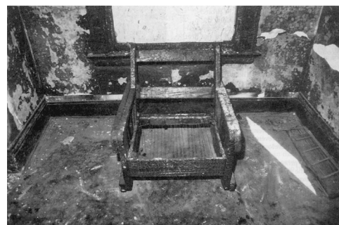
FIGURE 6.15.2.1 Photograph on Top, Showing Protected Area; Photograph at Bottom, Showing How the Chair Was Positioned During the Fire.
