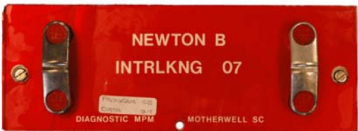
Westinghouse Diagnostic MPM Memory Module
