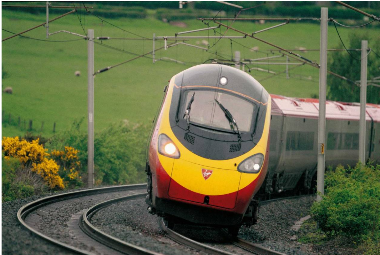
Figure 1 - Electric train and AC overhead line equipment
