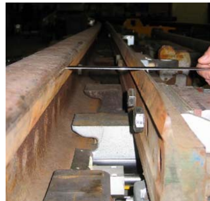
Figure 4: Measurement of Switch Rail Toe Travel
