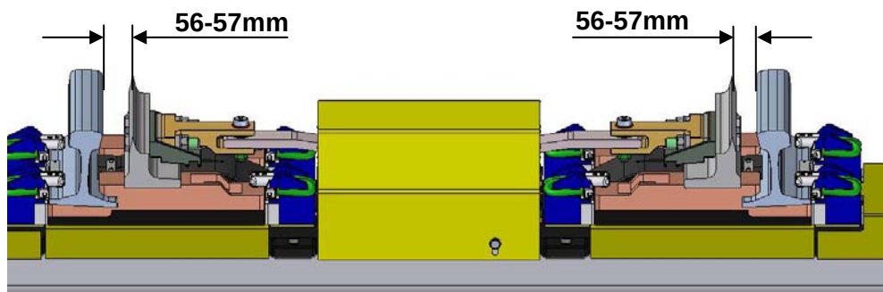
Figure 6: Switch Toes at Mid-Position (UIC54 & RT60)
