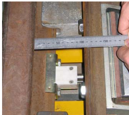
Figure 4: Measurement of Switch Rail Toe Travel
