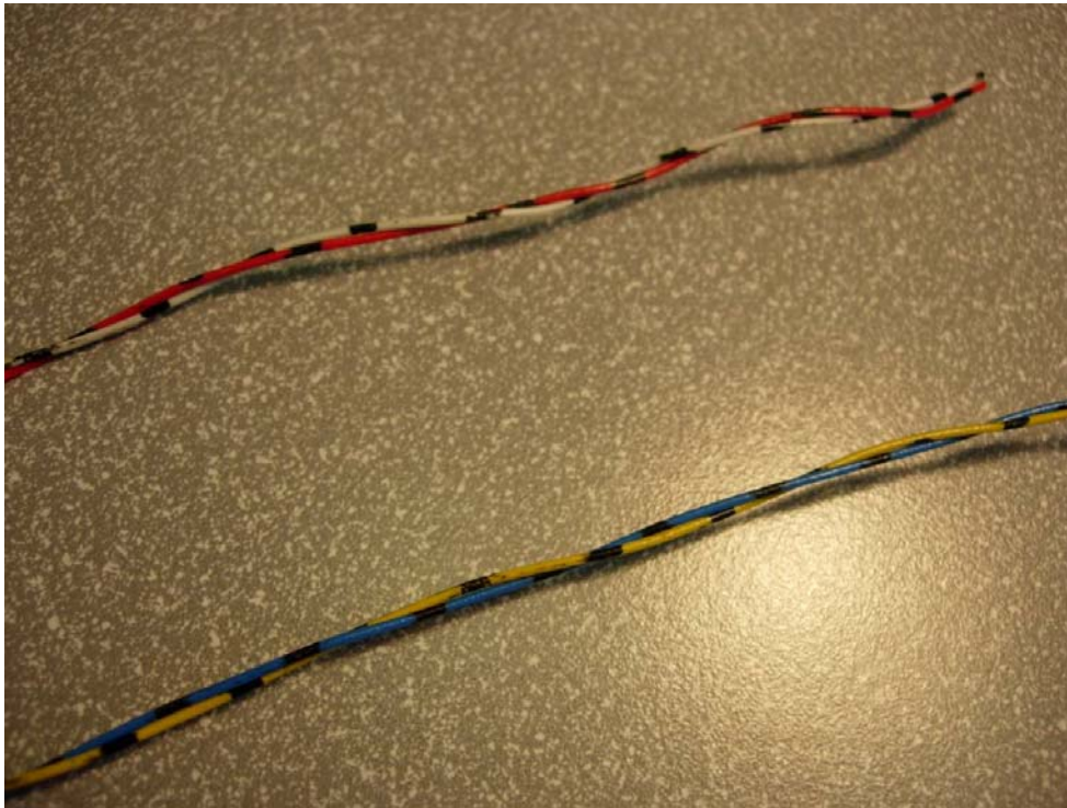
Figure 1: Banding on jumper wires
