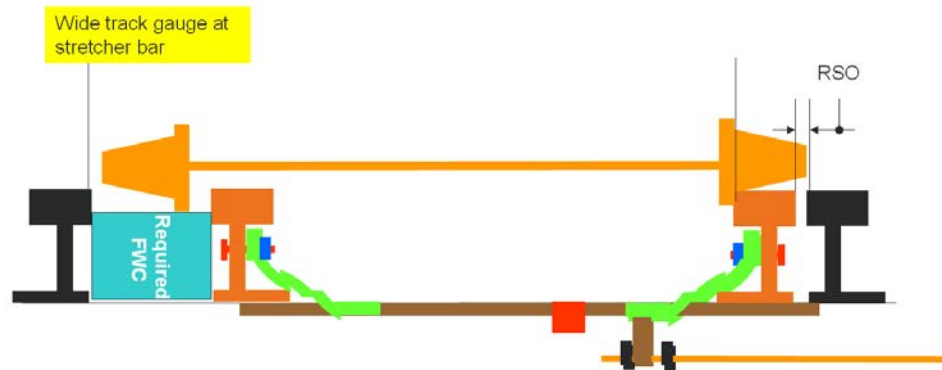
Figure 2c – With Required FWC FBC cannot occur even with wide track gauge
