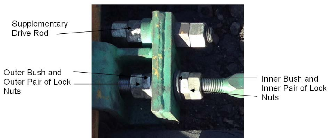
Figure 19 – Fitted pair of hard lock nuts
