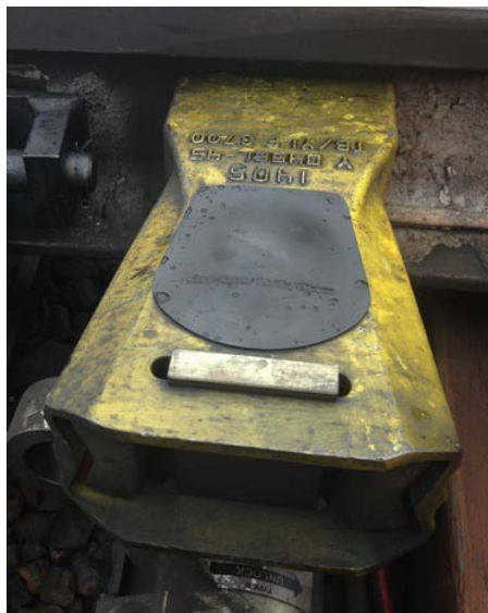
Figure 1 - Web Mounted Motion Units fitted to switch diamonds
