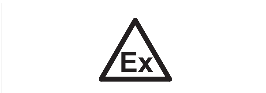
Figure 3 Warning sign for areas where explosive atmospheres may occur
