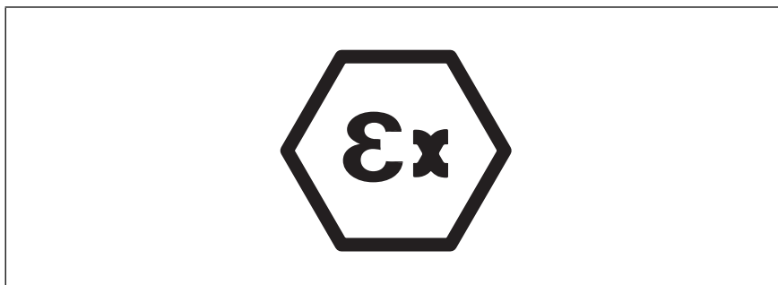
Figure 2 ATEX logo indicating that equipment is suitable for use in explosive atmospheres
