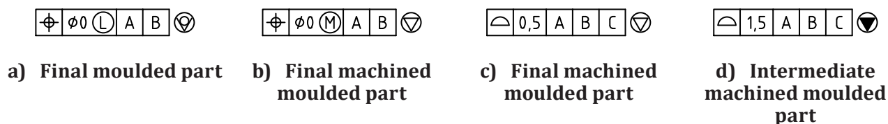
Figure 12 — Examples of geometrical tolerances with datum references
