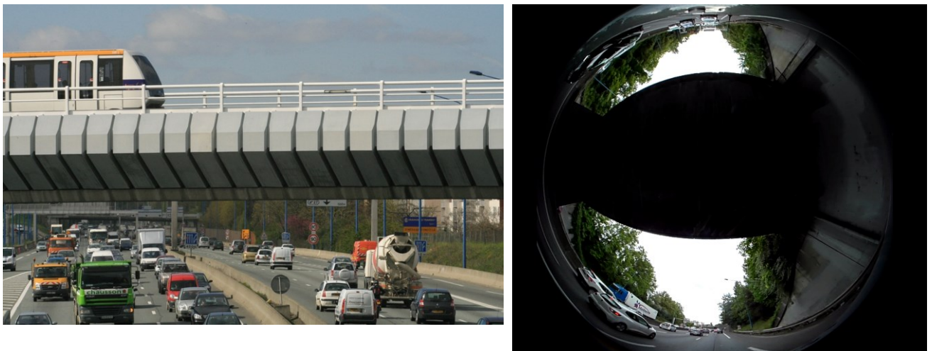
Figure 7 — Time spent under a bridge depends on traffic jam, and impacts positioning performances
