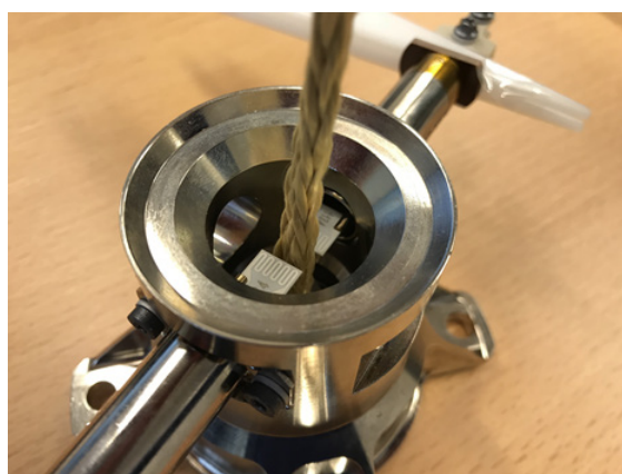
Figure 5-5: Thermal knife (with thermal heads visible)
