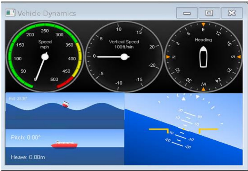
Figure 1 — Snapshot of GNSS simulator for antenna movement
