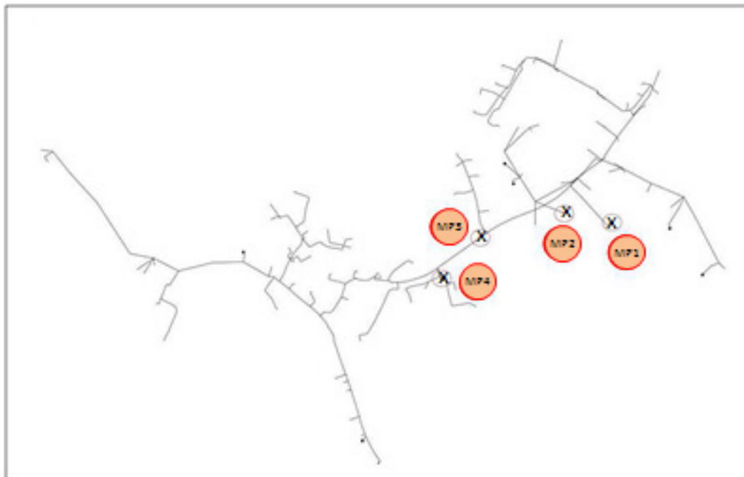
Figure 10 — Measurement of effects of a PV inverter
