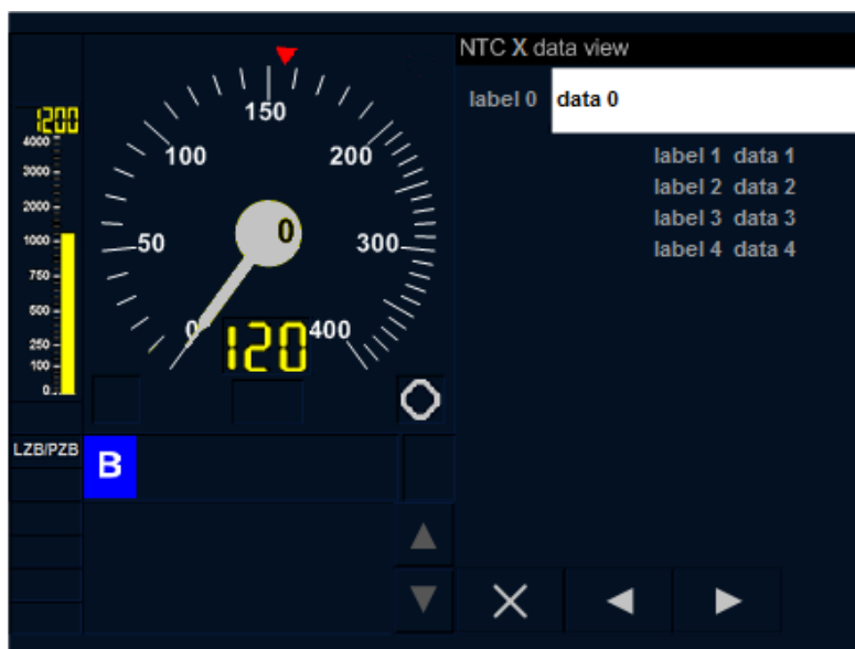
Figure A.7 — LZB/PZB data view window in touch screen technology
