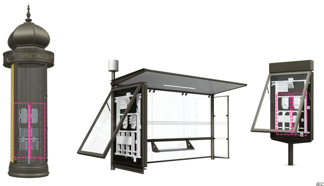
Figure 6 – Illustration of small cells integration in street furniture
