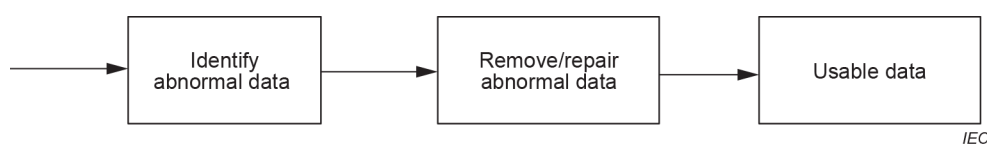
Figure 8 – Flowchart of abnormal power quality data identification
