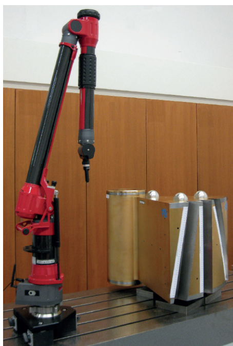
Figure 10 — Portable measuring arm with gear artefact
