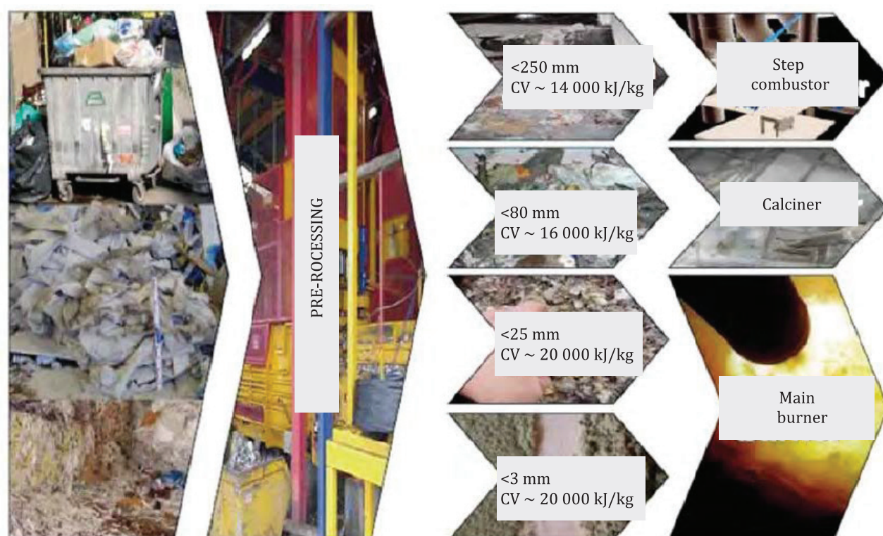
Figure 3 — Waste treatment and objectives with respect to the requirements of the burning process (adapted from [111] )
