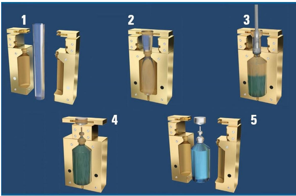
Figure3.1-1Diagrammatic Representation of the Open Parison BFS Process
