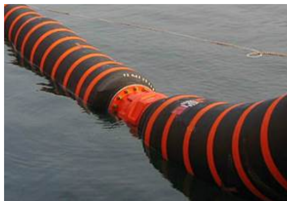
Figura 3 - Marine Breakaway Coupling (MBC) Instalada
