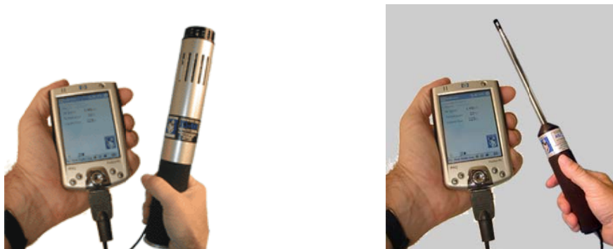
Figure 1: Examples of IAQ direct reading equipment
