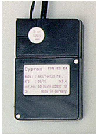
Figure 1: The CYPRES Processing Unit containing the battery, the pressure-measurement system and the processing electronics.
