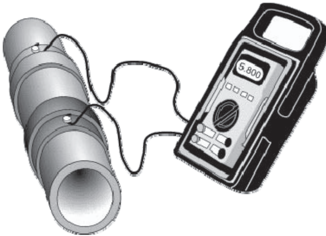
Figure 6 Typical Electrofusion Control Box and Leads with Clamps and Fittings
