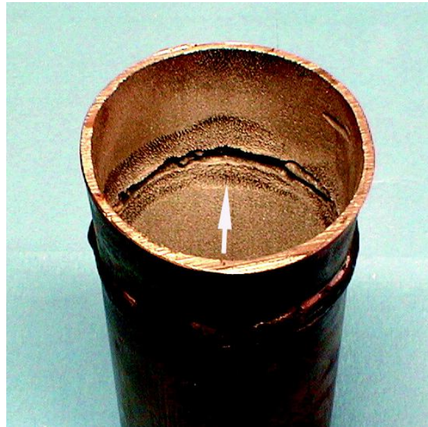
Figure 1. Carbon steel pipe butt joint weld showing severe internal corrosion of weld root and heat affected zone.
