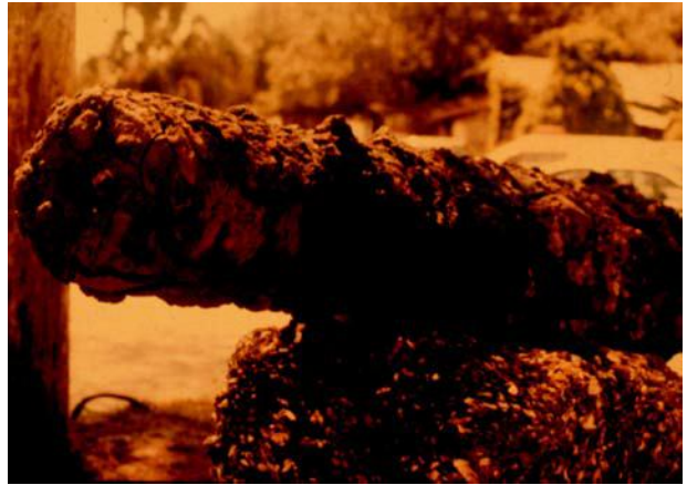
Figure 4. Severe general corrosion of a very old cast steel cannon barrel recovered after many years of being submerged in seawater. Note heavy scale of iron oxides that have completely filled the cannon bore.
