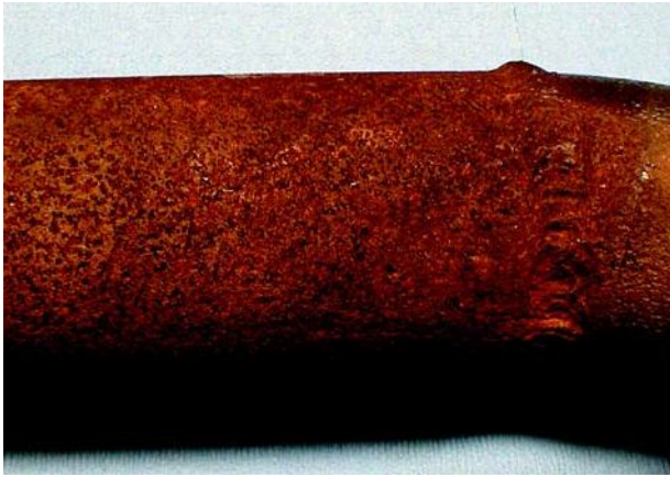
Figure 5. A carbon steel piping exterior showing moderate general corrosion of the pipe exterior and butt joint weld.
