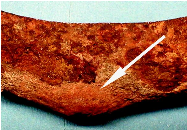
Figure 6. Bulge in boiler tube caused by loss of wall thickness by general corrosion and internal pressure on the thinned pipe wall.
