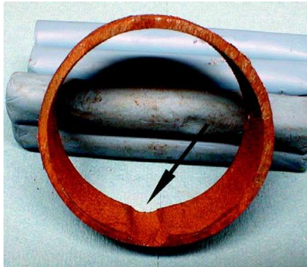
Figure 3. Pipe section showing localized corrosion of longitudinal seam weld.
