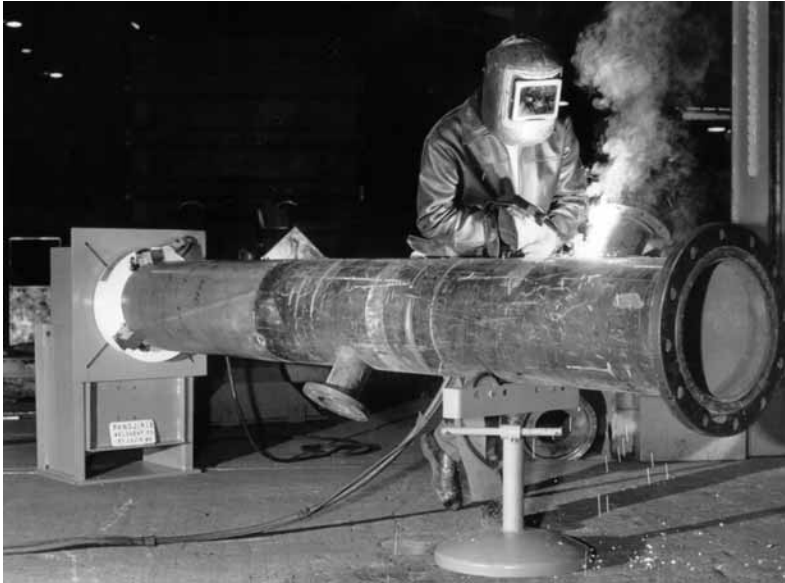
Figure 7—Use of a Three-Jaw Self-Centering Chuck
