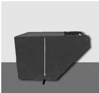
Figure 4A—Finding the Center of Gravity of Large Workpieces by Balancing them on a Pipe
