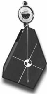
Figure 5A—Finding the Center of Gravity and Weight of a Workpiece using a Hoist and Scale
