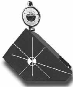
Figure 5A—Finding the Center of Gravity and Weight of a Workpiece using a Hoist and Scale
