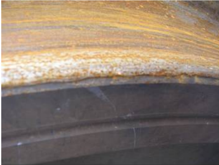
Figure 2 Photograph of tread roll-over
