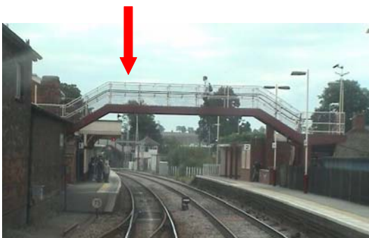
Figure 9 Visibility factors: station furniture can obscure signals
