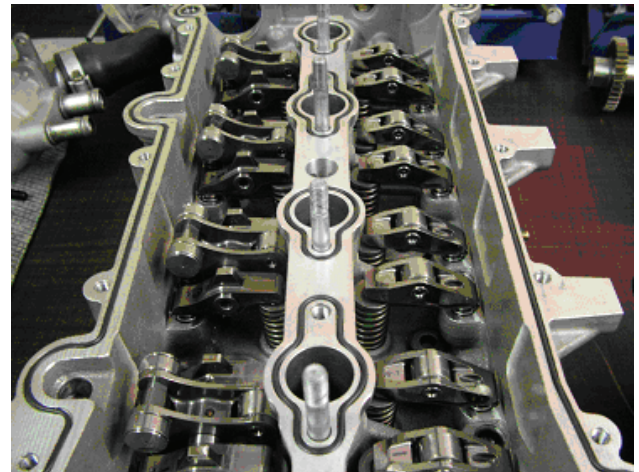
Figure 11: Shows the open cylinder head structure.
