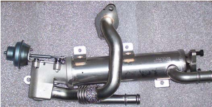
Figure 3. Bypass HPL EGR cooler (provided by Dayco USA)
