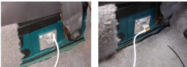
Figure 10. X-axis Accelerometers Mounted on “B” Pillars (left shown) for Frontal and Rear Tests; Y-axis Accelerometer Mounted on Left “B” Pillar for Side Tests.
