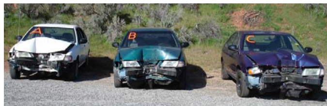
Figure 1. Nissan Sentra Frontal Impacts at 54 mph, 32 mph, and 21 mph with \Delta V 's of 20 mph, 13 mph, and 7 mph. (Matching these speeds to Tests "A", "B", and "C" cannot be based upon observed damage because the damage is essentially the same for each.)
