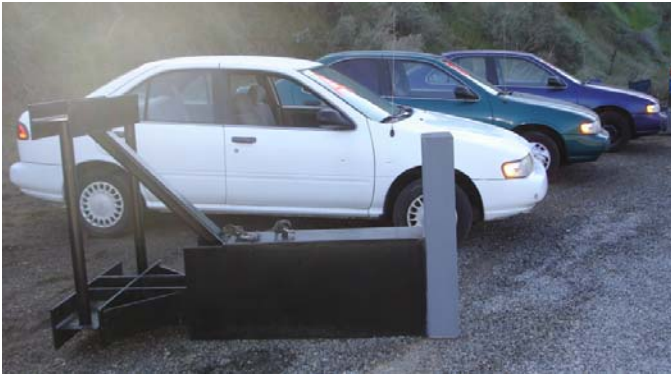
Figure 4. Impactor Used in Test Series “A”, Prior to Mounting on the Massive Moving Barrier.
