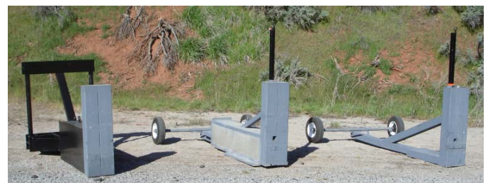
Figure 3. Impactors for Test Series “A”, “B”, “C”, in Order Left to Right.
