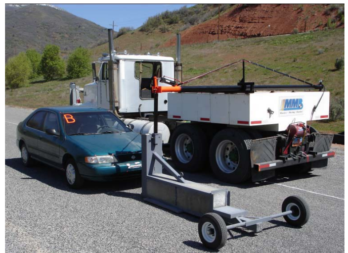
Figure 8. Towing Impactor into Stationary Target.
