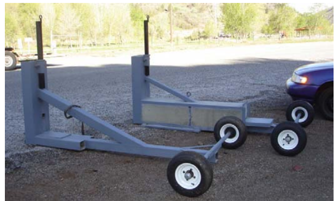
Figure 7. Side View of the Light Weight “C” Series Impactor (Foreground) and the Middle Weight “B” Series Impactor.
