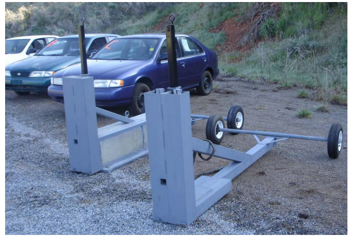
Figure 6. Impactors Used in Test Series “B” and “C”.
