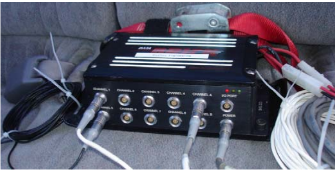
Figure 11. Data Collection Module, “Data Brick”.
