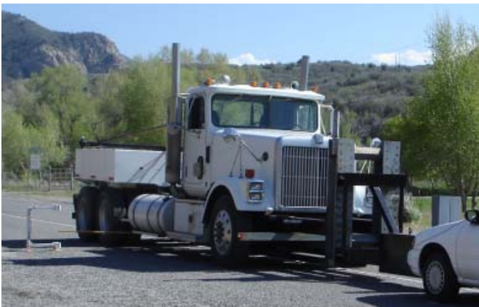
Figure 5. Massive Moving Barrier Used in Test Series “A” and as a Tow Vehicle in Test Series “B” and “C”.
