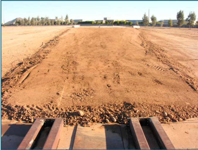
Figure 2: Photograph depicting a typical test surface. In the foreground the ends of the “snubber” tubes are visible. The snubber tubes approximate the stopping point for the portion of the dolly under the left-side tires.
