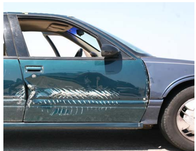
Figure 16. Test 2 – Right front door post test.
