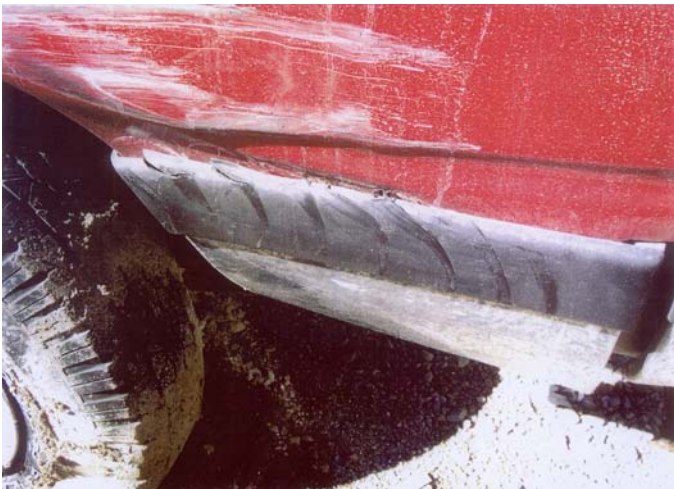
Figure 7. Lug contact mark on lower left rear trim.
