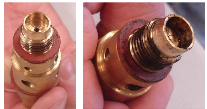
Figure 4. Photographs of the probe after one run (left) and after all testing was completed (right)
