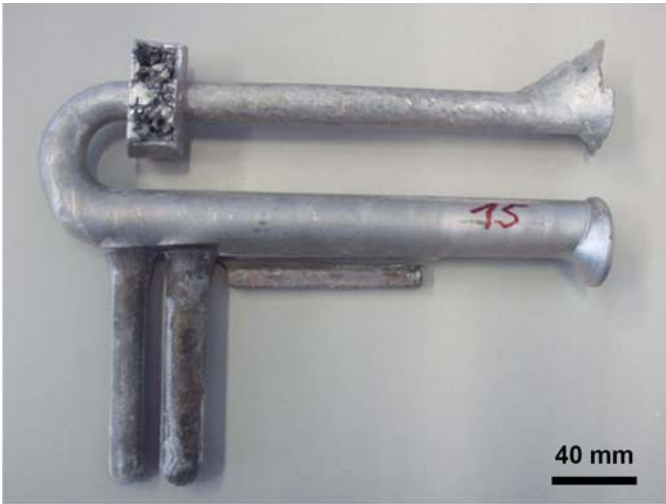
Figure 2. Permanent-mould cast AM-SC1 test specimens, with runner system.
