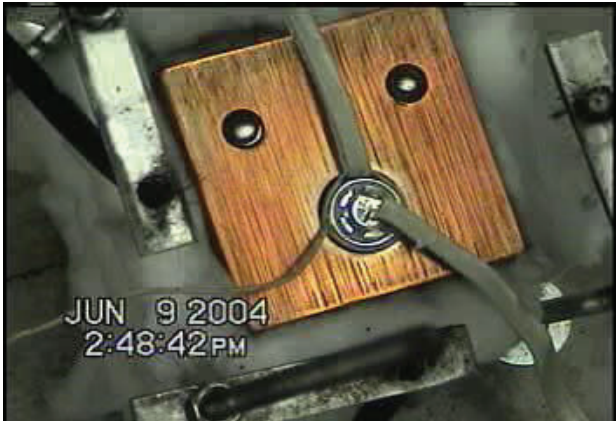
Figure 4. Thermal ramp apparatus with 18650 cell in center.
