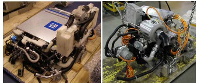
Figure 6: Sequel's fuel cell stack module and front electric traction system
