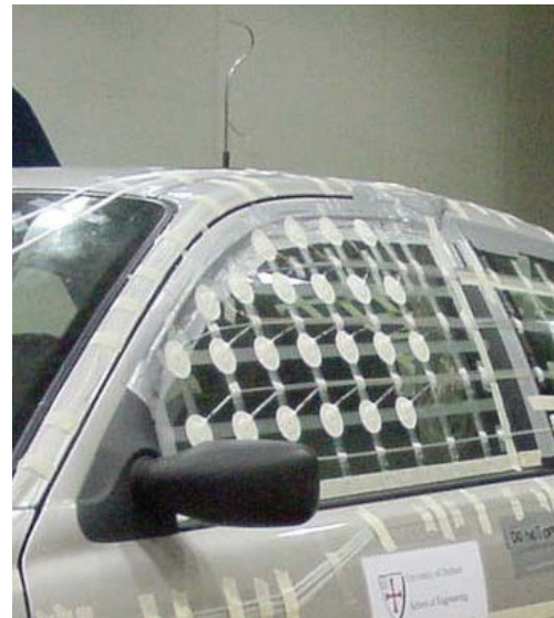
Figure 4: Test vehicle with pressure tappings
