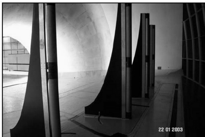
Fig. 2: The Pininfarina Turbulence Generation System (Cogotti, 2003)
