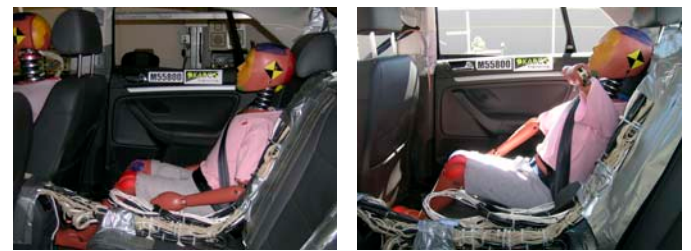
Figure 9. 10-year-old Child Hybrid III Dummy without booster in Pre/Post crash (5374)
