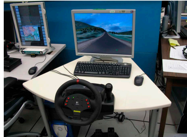
Figure 6. Secondary (wingman) crewstations. (left) Secondary gunner's station consisting of one touch screen display and a joystick controller. (right) Secondary driver's station consisting of a day-view display, a steering wheel, and two pedals.
