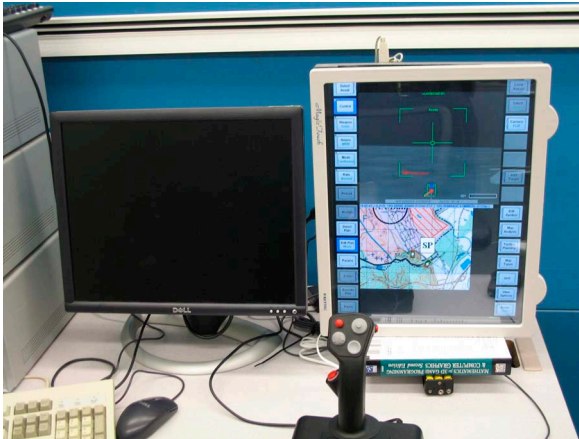
Figure 6. Secondary (wingman) crewstations. (left) Secondary gunner's station consisting of one touch screen display and a joystick controller. (right) Secondary driver's station consisting of a day-view display, a steering wheel, and two pedals.
